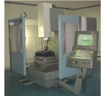
3-axis ultrasonic machining facility
